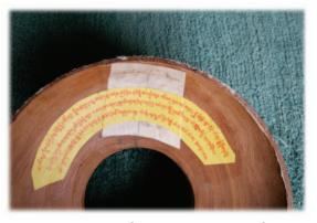
Large epoxy patch over serious crack
